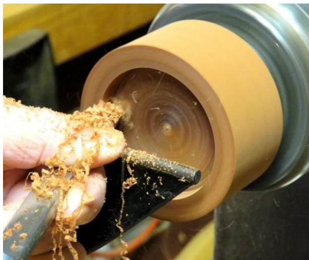
Figure 3- Cutting the lid mortise
