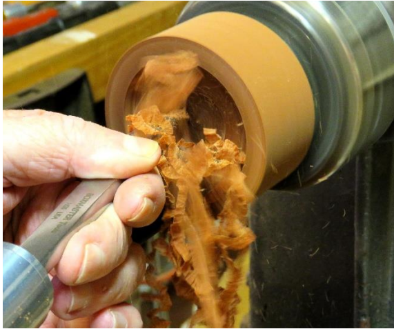
Figure 4- Shaping the interior dome
