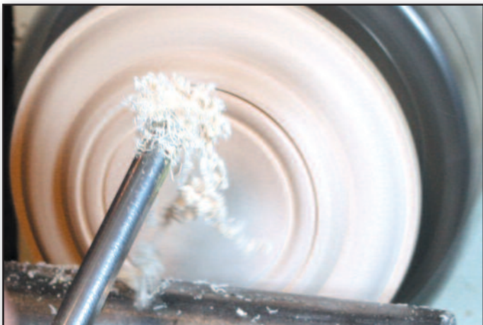
This end-grain beading was done with the 1/4" beading tool. Notice the fine ribbons on the end of the tool.
