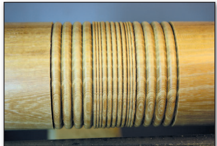
These beads were turned with the 1/16", 1/8" and 1/4" beading tools on osage orange. Consistent spacing was relatively easy with just a few minutes practice.
