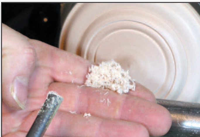
This is an example of the fine ribbons possible with the 1/4" beading tool.
