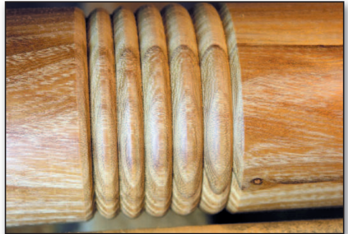
These beads were turned with the diamond (teardrop) tool on osage orange.
